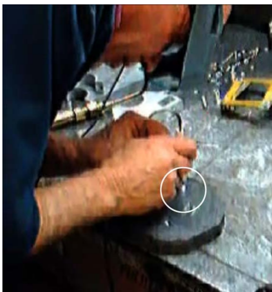
Fig. (22). Applying a small torch to a minute red chip (left), followed a few seconds later by ejection of material, producing a horizontal orange streak running toward the operator's hand (right). (Frames from video of this flame/ignition test).
